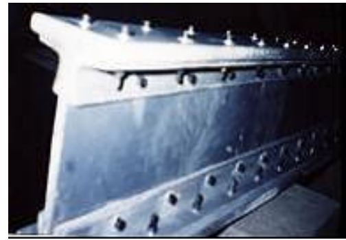
(a) Bolted I-beam
